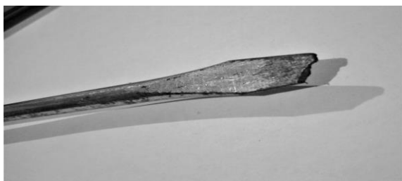
Chipped Flat screwdriver head
