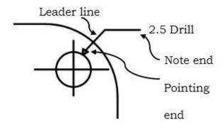
5. Arrowheads indicate the direction in which the value applies. They are drawn in freehand either on one or two strokes.
