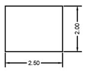
The purpose of dimensioning is to provide a clear and complete description of an object. A complete set of dimensions will permit only one interpretation needed to construct the part. Dimensioning should follow these guidelines.
