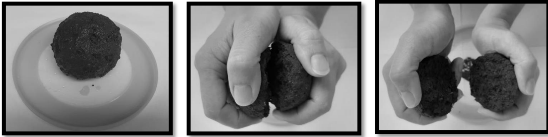
Figure 4. Pulling apart to break the ball of soil.
